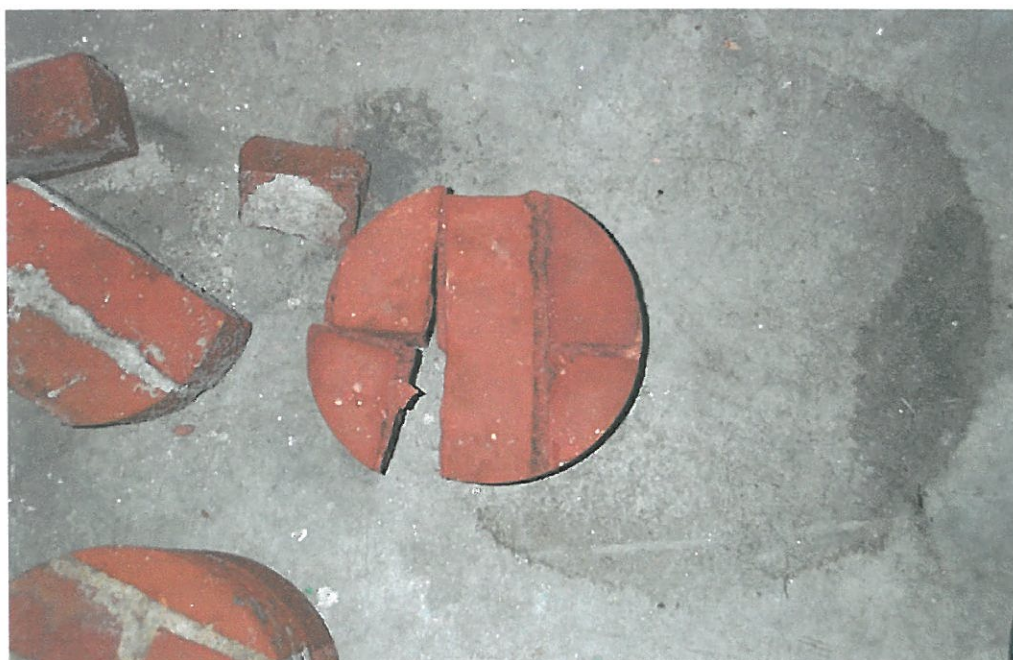
Brick core at wall mid-height. Note deteriorated mortar.
